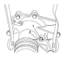
even with the bottom of the side fill hole. Refer to the Gearcase Specifications Chart on page 80 for recommended lubricants, capacities and torque specifications. See page 114 for the part numbers of Polaris products.
